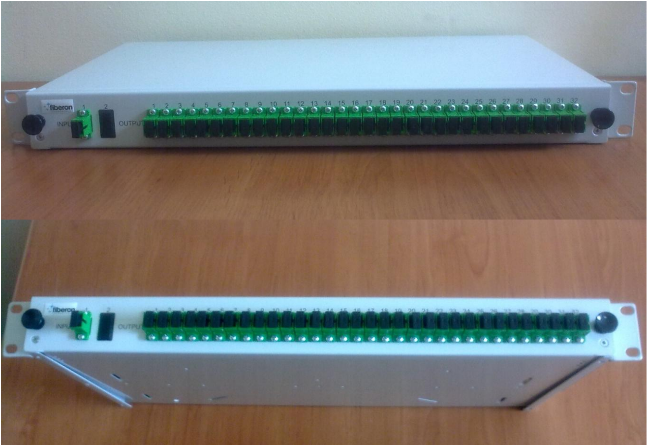
Panel 19"/1U ze spliterem PLC 1x32 SC/APC SM
